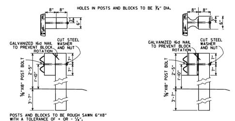
PLASTIC BLOCKOUT CONNECTIONS WOOD BLOCKOUT CONNECTIONS DETAILS OF WOOD LINE POST CONNECTIONS (W-BEAM)
