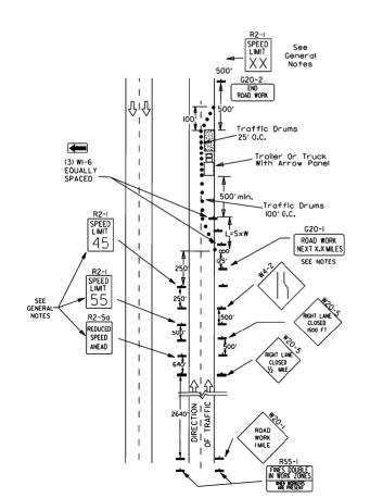
Typical application - construction operations of intermediate to long term duration on a 4-lane divided roadway where half of the roadway is closed.
