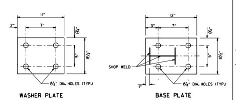
Note: Bolts, nuts, washers and plates shall be galvanized in accordance with Section 807 of the Standard Specifications.
