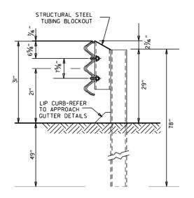
THRIE BEAM RAIL WITH STEEL TUBING BLOCKOUT AND STEEL POST POSTS I-7
