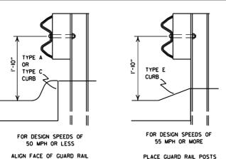
PLACE GUARD RAIL POSTS AGAINST BACK OF CURB. WITH FACE OF CURB.
