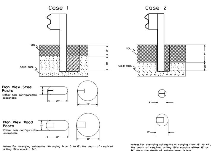
the depth of required drilling (B) is equal to either 12" or 44" minus the depth of soil whichever is less.
