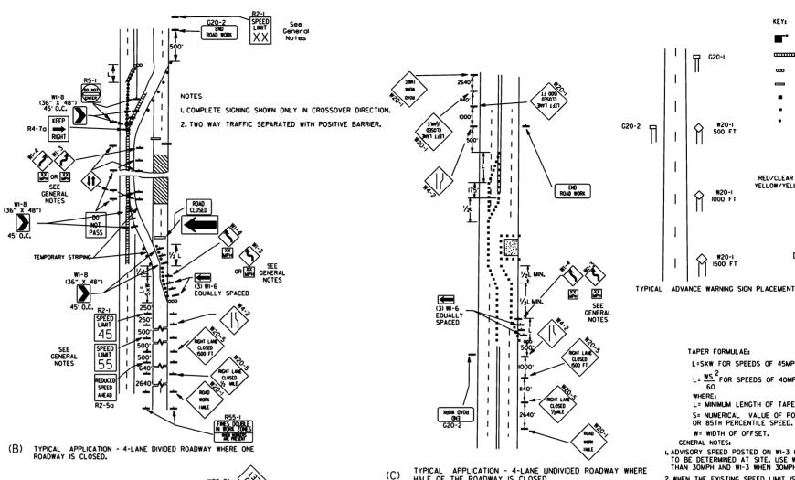
ROAD WORK CHANNELIZING DEVICES SEPARATE WORK AREA FROM TRAVELED WAY (OPTIONAL) TRUCK MOUNTED ATTENUATOR ROAD WORK END G20-2 ROAD WORK I. FLOOD LIGHTS SHOULD BE PROVIDED TO MARK FLAGGER STATIONS AT NIGHT AS NEEDED. END. 2. IF ENTIRE WORK AREA IS VISIBLE FROM ONE STATION, A SINGLE FLAGGER MAY BE USED. 3. CHANNELIZING DEVICES ARE TO BE EXTENDED TO A POINT WHERE THEY ARE VISIBLE TO APPROACHING TRAFFIC. 4. AUTOMATED FLAGGER ASSISTANCE DEVICE (AFAD) OPTIONAL. REFER TO MUTCD. WORK
