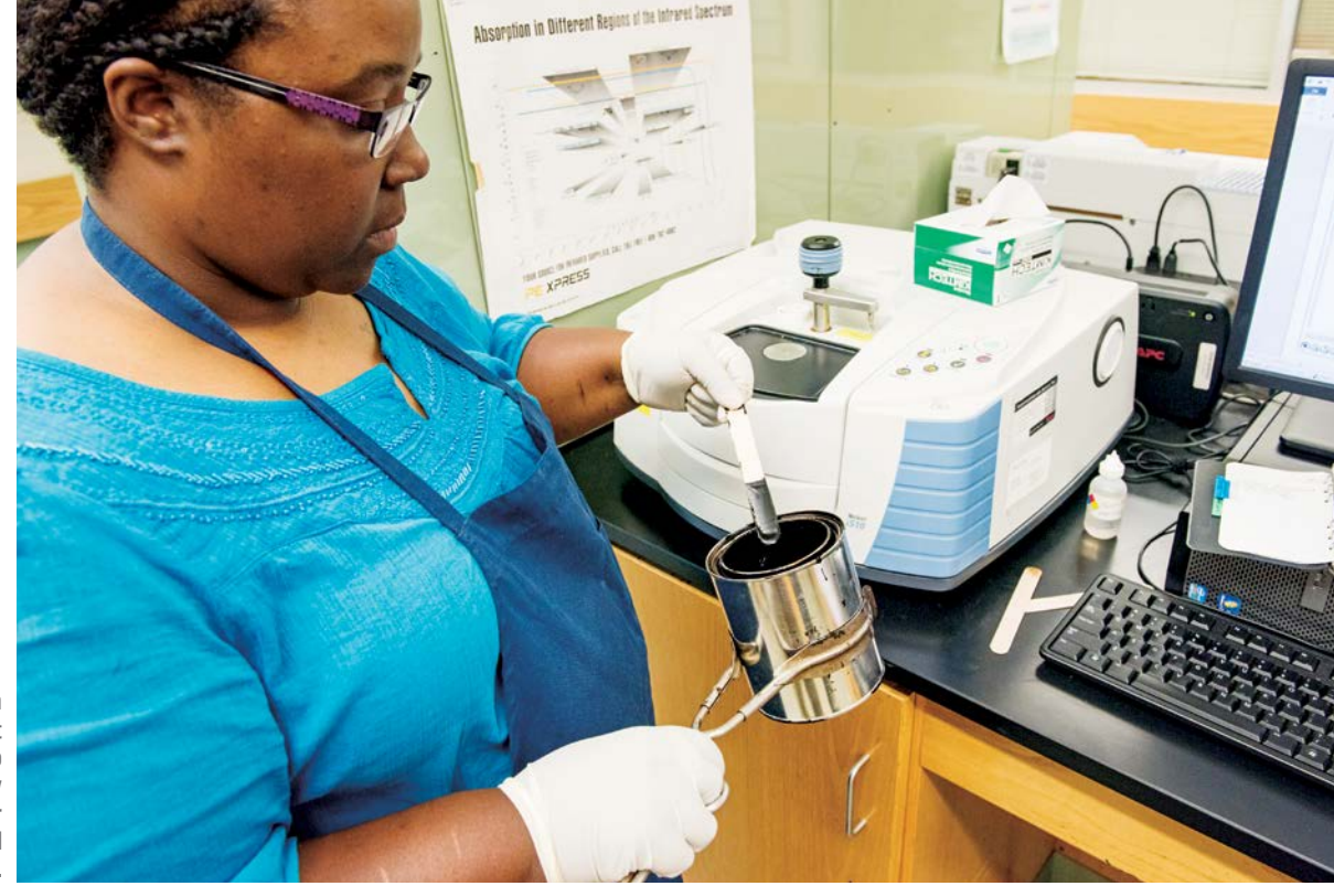
Cynthia Pearson tests asphalt polymer content to observe its elasticity using a Fourier Transform Infrared Spectrometer.
