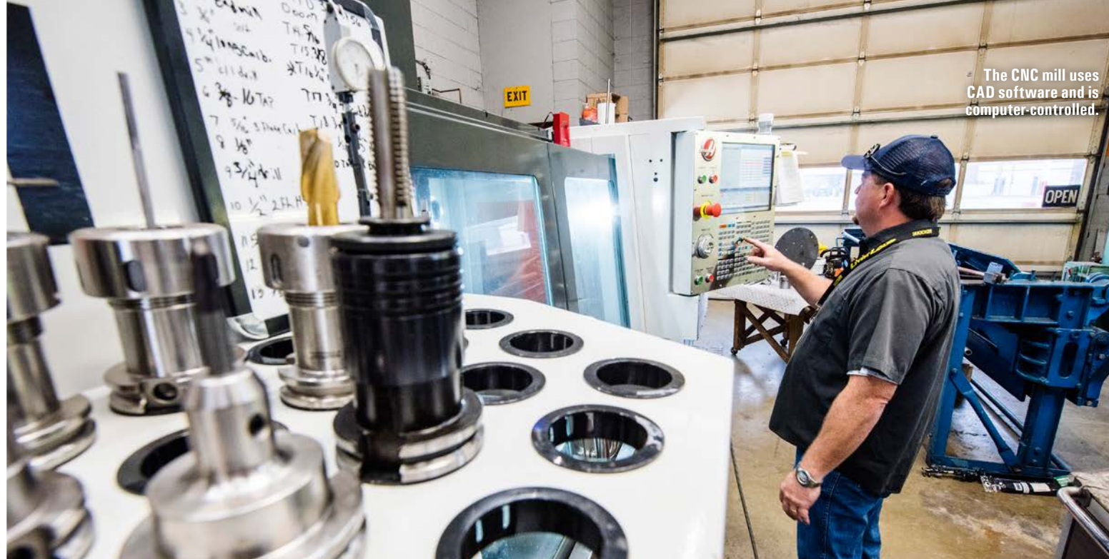
The cutter that the machine has in the spindle will carve through the material and create the intended shape.
