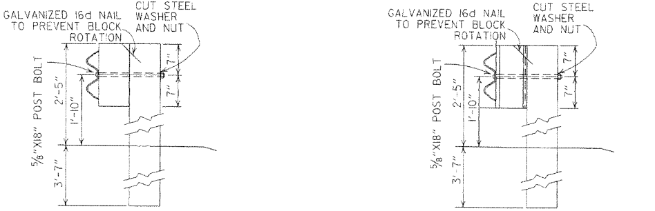
WOOD BLOCKOUT CONNECTIONS PLASTIC BLOCKOUT CONNECTIONS DETAILS OF WOOD LINE POST CONNECTIONS (W-BEAM)
