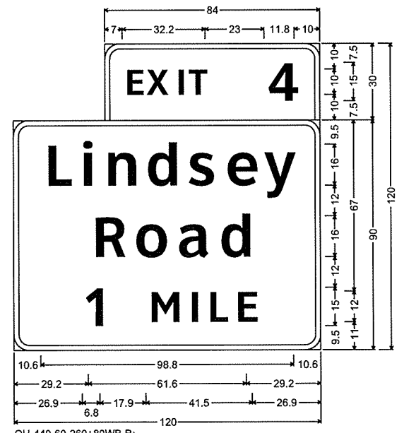
OH-440-60-260+80WB-B; 6.0" Radius, 2.0" Border, White on Green; [EXIT] ClearviewHwy-5-W; [4] ClearviewHwy-5-W; 6.0" Radius, 2.0" Border, White on Green; [Lindsey] ClearviewHwy-5-W; [Road] ClearviewHwy-5-W; [1] ClearviewHwy-5-W; [MILE] ClearviewHwy-5-W;
