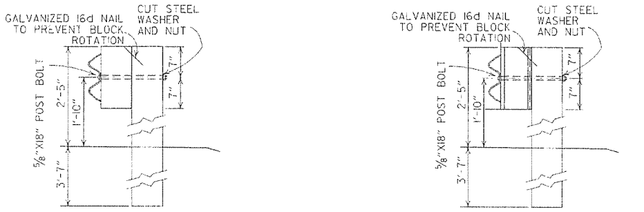
POSTS AND BLOCKS TO BE ROUGH SAWN 6" X 8" WITH A TOLERANCE OF + OR - 1/4". WOOD BLOCKOUT CONNECTIONS PLASTIC BLOCKOUT CONNECTIONS DETAILS OF WOOD LINE POST CONNECTIONS (W-BEAM)
