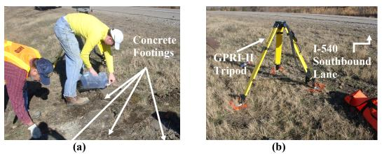
Figure 2.8. a) Placing concrete footings for GPRI-II at the Southbound viewpoint at the calibration site, and b) tripod of GPRI-II anchored at the Southbound viewpoint near Chester, Arkansas..
