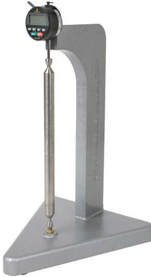
Figure 3.4 Length Comparator with Digital Indicator ( www.humboldtmg.com )
