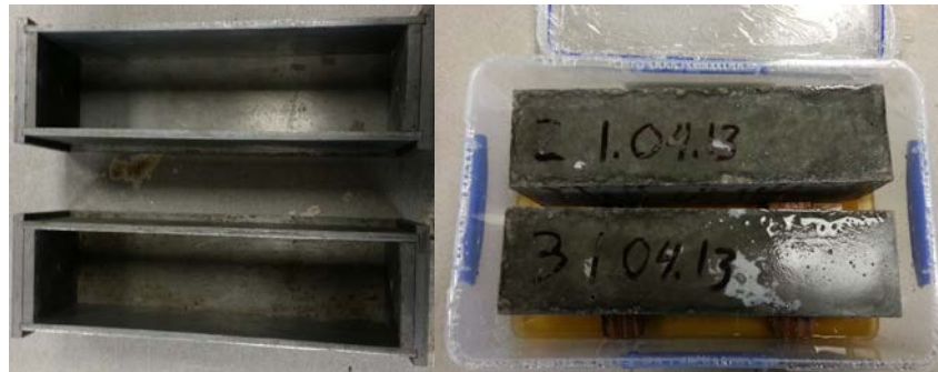
Fig. 3.3.2-1 Typical CPT prism molds (left), and storage containers (right).
