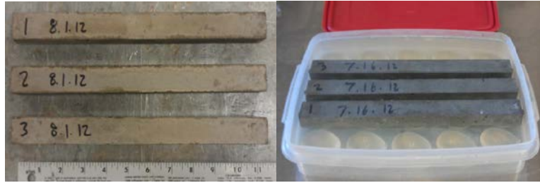
Fig. 3.3.1-2 Mortar-bars (left) and mortar-bar in storage container (right).
