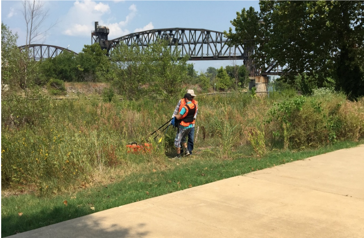
Figure 4.1.31 - Thick bushes/weeds made the survey extremely difficult due to the large size of the 200 MHz antenna.
