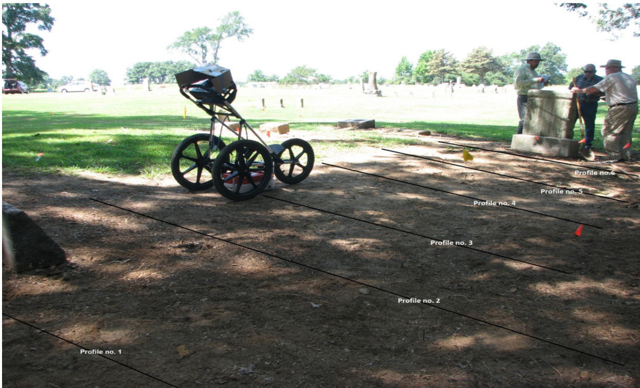
Figure 4.2.2. Photograph at Area 1 showing location of profiles 1 – 6 and the GPR cart.
