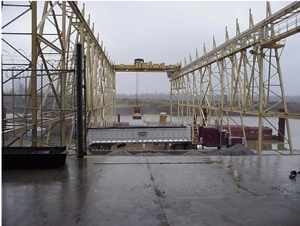
Truck being loaded from a barge
