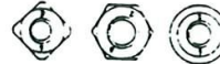
METRIC SQUARE HEX AND ROUND HEX NUTS DEPRESSED LETTERS AND CLASS NO.
